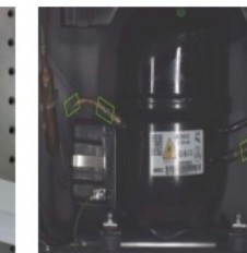
(k) 管状焊点检测[42]
